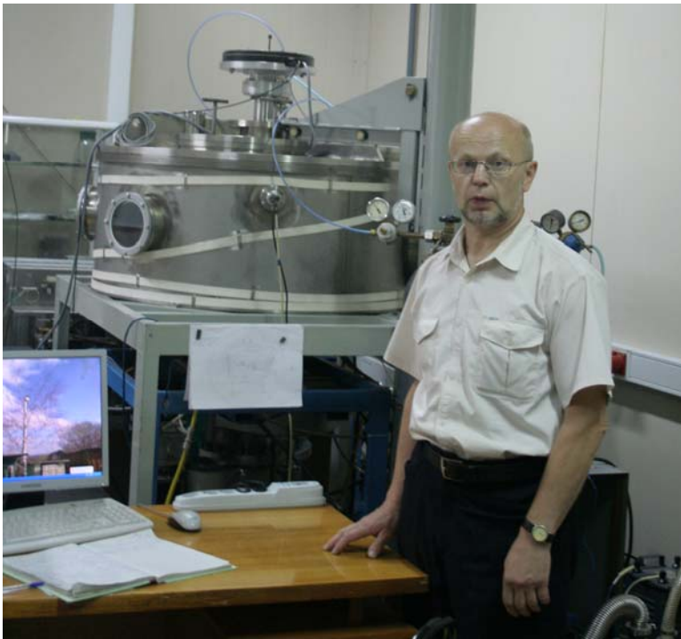
Technological installation with six magnetrons for MLSs deposition. In the foreground shown “owner” of this installation B.A. Volodin.
