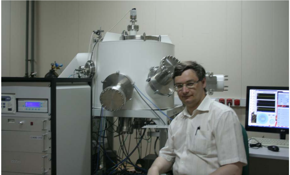
The multipurpose stand for MLS deposition by magnetron and ion-beam sputtering methods, including an opportunity of layer surfaces polishing by low energy ions.
