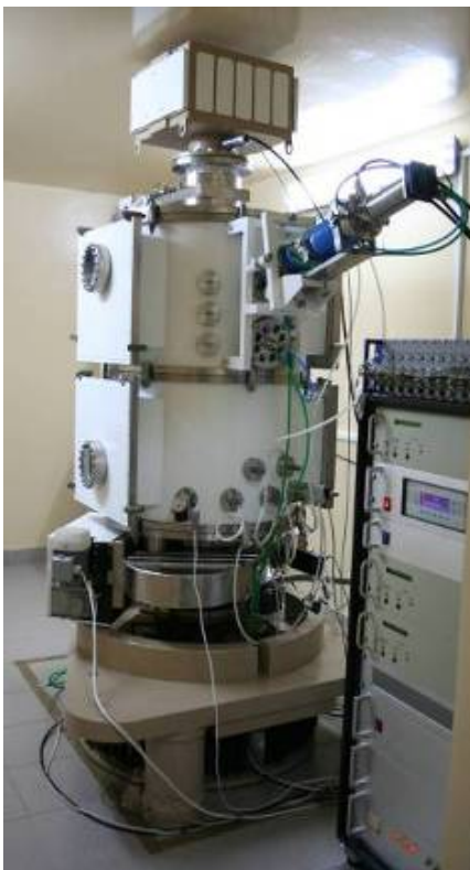
Photo of the nanolithographer-multiplier developed in IPM RAS.
