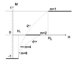
FIG. 3. The steps on the magnetization curve corresponding to simple superstructures  $(m=2^k)$  with one reversed magnetic moment per period. Magnetization of the corresponding step is  $M = (2-m)/m = -1 + 1/2^{k-1}$ .
