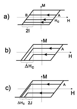
FIG. 8. The hysteresis curve in the mean field approximation. (a) for the system with interaction with the same coercivity of any magnetic moment; (b) for the coercivity dispersion (uniform distribution of the coercivity) and without interaction; and (c) for the system with both interaction and coercivity dispersion.
