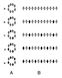
FIG. 1. The reversal process in the cyclic system of eight magnetic moments and the corresponding superstructures in the infinite system. White arrows are for nonreversed magnetic moments; black arrows denote the already reversed ones. The external field increases from (a) to (e). (A) The reversal process in the cyclic system of eight magnetic moments and (B) the corresponding superstructures in the infinite system.
